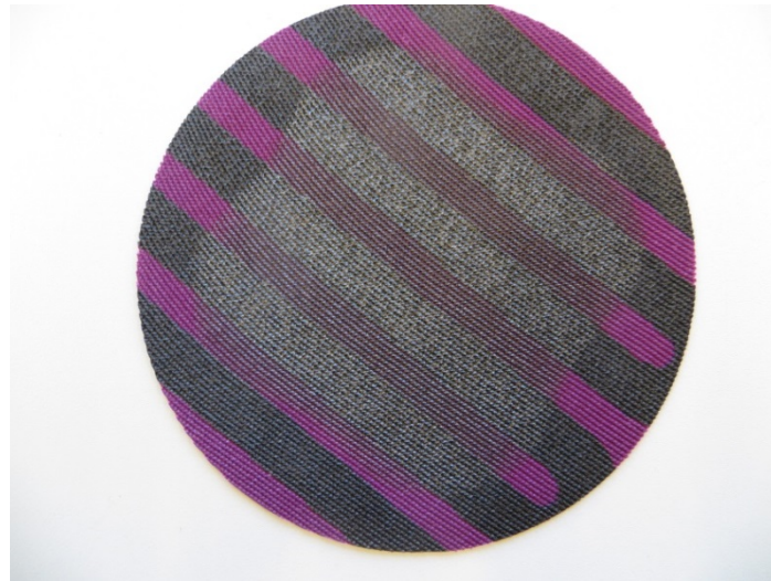
Image 1: meander of printed carbon in after 5,000 Martindale cycles.
