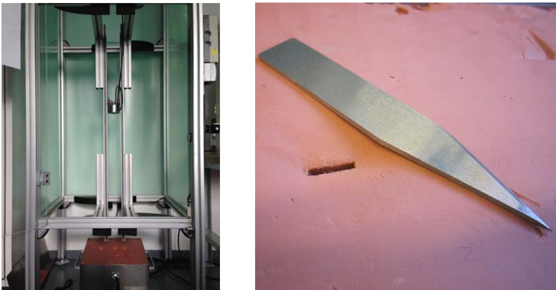
Fig. 1. Stab resistance test stand with rails leading the falling weight with the blade attached, electromagnet holding the falling weight and plasticine box (left panel), blade according to VPAM test instruction with typical cut in the plasticine.
